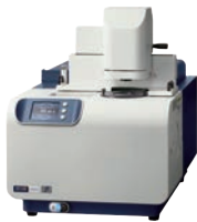
HITACHI熱示差掃描分析儀 (DSC) NEXTA® DSC600 & DSC200
